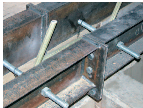
3 - Compression table lined with supporting ironwork for self-bearing floor
